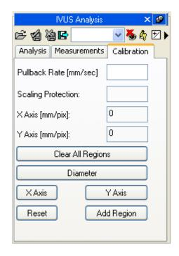
If no information appears then the image needs a calibration. This operation must be executed very carefully because all subsequent measurements strictly depend on the calibration procedure.
