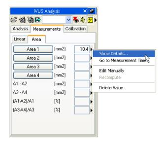
By clicking on the little arrow and then on *Show Details*, a window will be displayed in which all the samples taken for that item are shown together with the average and the standard deviation.
