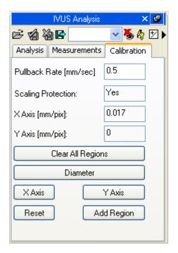
In the absence of a correct calibration or pullback velocity all measurements are invalid.
