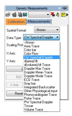
Next, establish (using the X axis and the Y axis) the calibration values to be assigned to the image. For instance, in case of a Doppler image, assign a time value on the X axis and a speed value on the Y axis. For 2D images, which have the same unit of measurement for both axis, it is also possible to calibrate both axis at once with a single diagonal segment using the *Both* button.
