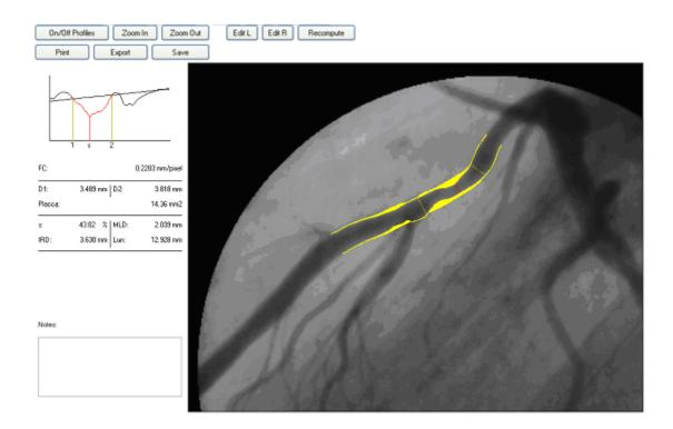
The image and the borders are zoomed to better visually verify the correctness of the measure. The coronary borders are displayed in yellow on the original image. The program also identifies the stenotic point of the vessel and the estimated normal profile. The former is indicated by a red segment perpendicular to the centerline whereas the latter is indicated in yellow. The region between the measured coronary borders and the normal profile is also filled with a yellow color.
