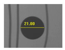
On the image, click the left mouse button at one end of the segment to be measured and then release it. By moving the mouse it is possible to trace the desired segment. Click the left mouse button once again, the segment can be fixed. The related calibration factor will be automatically calculated and displayed in the suitable edit control. Alternatively, by right clicking the mouse button during segment tracing, the operation can be cancelled.
