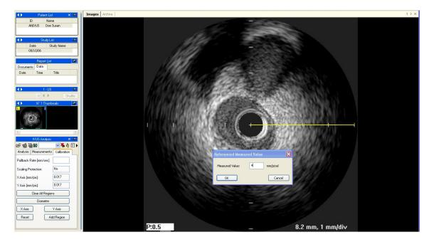
It is also possible to set the IVUS image diameter by clicking separately on the *Diameter* button. If such operation is not executed, the diameter is the greater value between the one identified by the X and the Y calibration.
