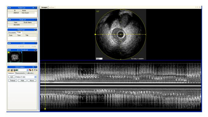
If the DICOM object is an IVUS sequence, you may perform a longitudinal reconstruction in real time during loop playback by clicking the *ILD* button. The position and the image dimension depend on the drop-down window near the *ILD* button.
