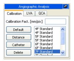
The calibration on a known catheter size can be carried out by clicking the *Catheter* button in the *Calibration* tab. In the white frame, a list of names corresponding to the pre-set known catheters are shown. By default, the catheter most recently used is selected and emphasized in blue If needed, select a different one with the left mouse button.
