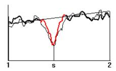
Moreover, with a double click on the graph, the program will display the densitometric analysis results. The previous geometric analysis is reported in underlay for a direct comparison. A further mouse double click will return to the previous results display.
